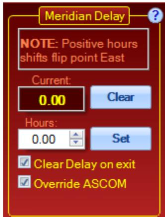
**Current:** The current meridian delay as polled from the mount. Note how this value changes at different declinations if APCC's Meridian Limits are enabled. This is the manifestation of the "dynamic meridian delay" described earlier.
