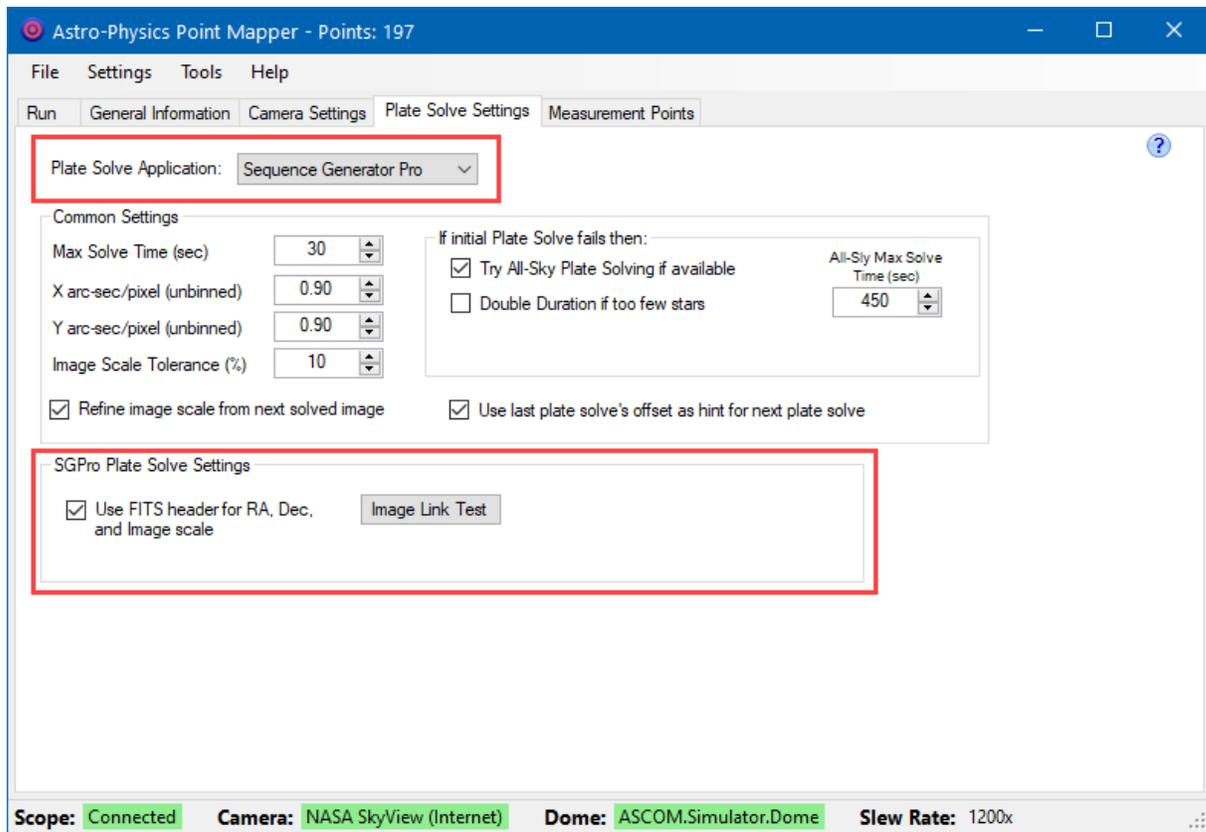
**Use FITS header for RA, Dec, and Image Scale:** Hints for position and image scale will be extracted from the image, if they are present.
