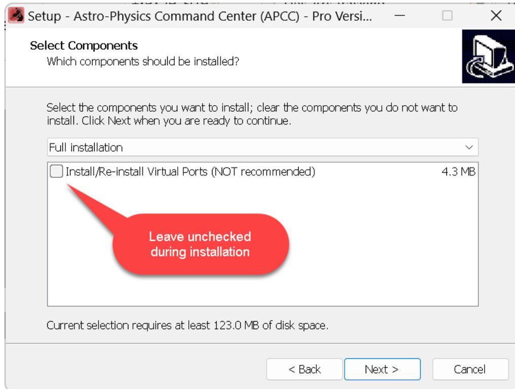
**IMPORTANT NOTE IF YOU INSTALL VIRTUAL PORTS:** Near the end of the software installation process, a black DOS-style Command window might open. **DO NOT** interfere with this command window! Don't touch anything on your computer, including the mouse or keyboard while this window is up. Doing so may cause a failure of the virtual port system. Please be patient!
