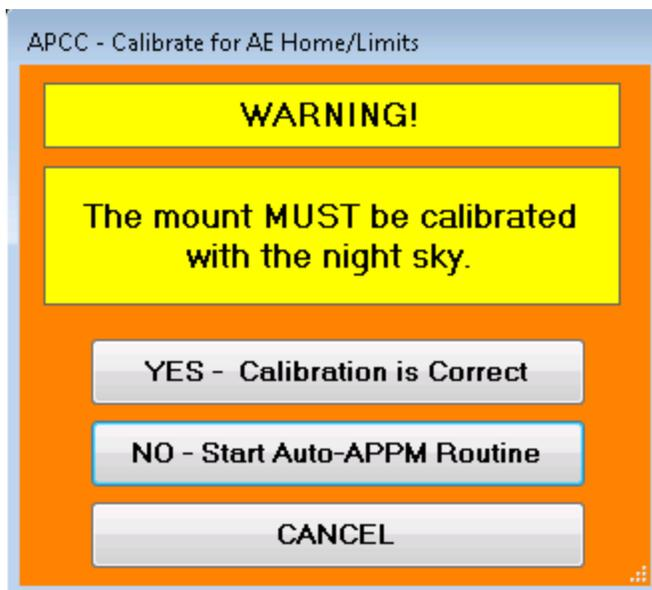
**YES - Calibration is Correct:** Click this button if the mount's calibration has been established, such as by doing a RECAL on plate solved coordinates.
