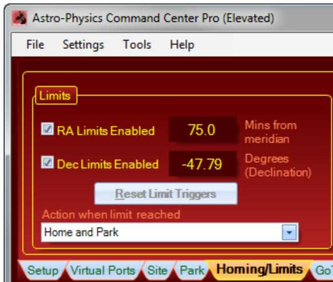
The Limits Box is where you enable or disable the limits you have configured. It is also where you set the action that will occur should you slew or track into a limit. To enable or disable the RA or Dec limits, simply check or uncheck the appropriate box.
