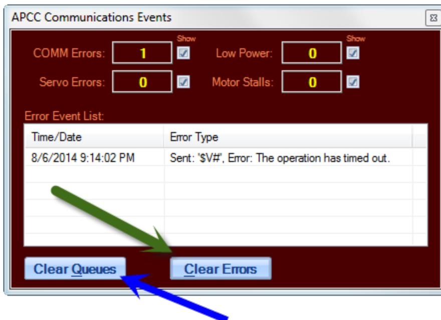
Click the **Clear Errors** button to clear the screen. When you close the window, the **COM Events** button will be grayed out again. The **Clear Queues** button may be needed if you have an Ethernet or Wifi problem that results in a large number of timeouts.
