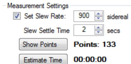
**Set Slew Rate:** If enabled the Slew rate value is used for slewing the mount. This overrides the settings in APCC and the driver.
