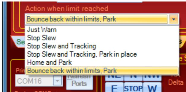
The options shown above are relatively self-explanatory, but there are a few things that we want to point out. In all cases, when a limit is reached, a warning box like the following will appear. The exact text of the warning will depend on the action-option chosen.
