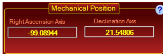
**Right Ascension Axis:** The internal mechanical angle (degrees) of the Right Ascension Axis. The mechanical position is relative to the established home position.
