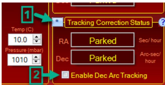
1. This button opens the Tracking Rate Tweak window. This allows you to see the commands sent to the mount as well as provides the ability to adjust the rates.
