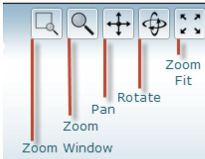
**Zoom Window:** Allows you to create an enlargement window for a specific portion of your 3D model. Left click on the icon to activate the crosshair. Scroll to move the crosshair to the desired starting position, click and draw a box, much like a crop tool in photo editing software. When you release your mouse button, the blue marked area will enlarge. To return your model to the default position, select the Zoom Fit icon.
