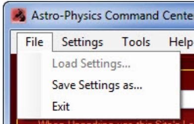
**Load Settings:** This will open a dialog window from which you can select a previously saved settings file. This menu item is only available (i.e. active) when APCC is not connected to the mount.
