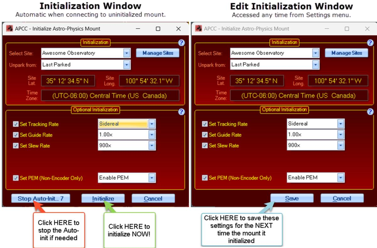
IMPORTANT: The window on the left above will NOT appear if you have already initialized the mount (including initializing the mount with another source, such as the keypad). Also bear in mind that the mount remains initialized until it is power cycled. Remote observatories that leave power on to the mount (not recommended in case of damaging lightening storms) will maintain an initialized state in the mount and will therefore not see this window upon startup of APCC.
