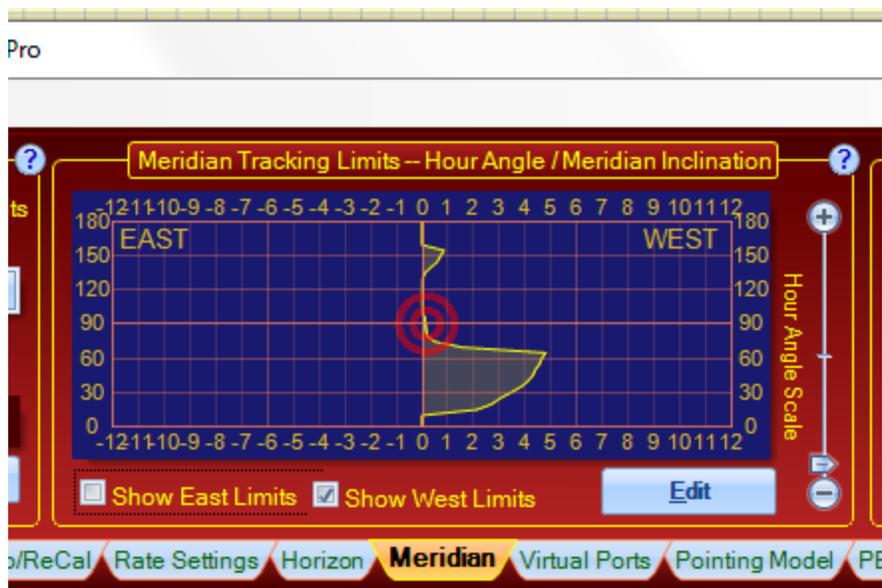
**Hour Angle Scale:** Allows you to magnify the hour angle values.
