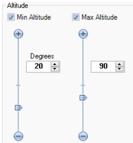
**Min Altitude:** when enabled no points below the minimum altitude are created. The checkbox **MUST** be checked for this limit to take effect!
