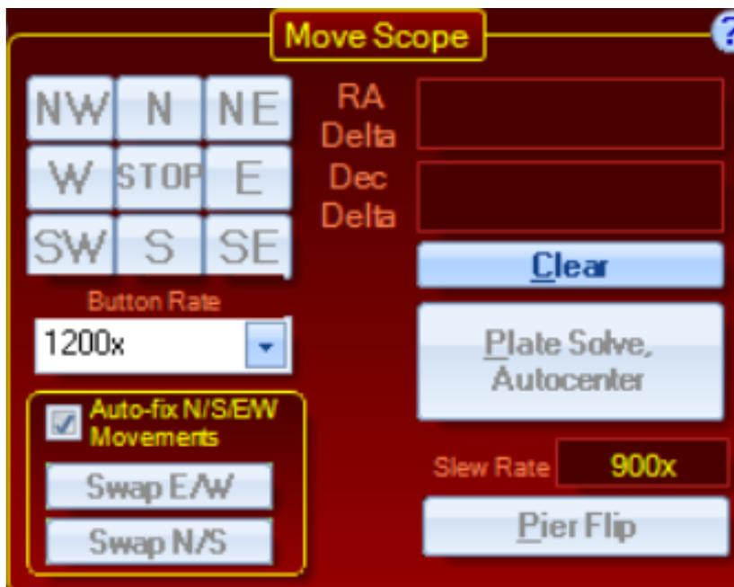
**N/S/E/W/NE/NW/SE/SW:** When pressed, the mount will move in the direction that the button indicates. The rate of movement will be defined in the *Move Button Rate* drop-down combo box.
