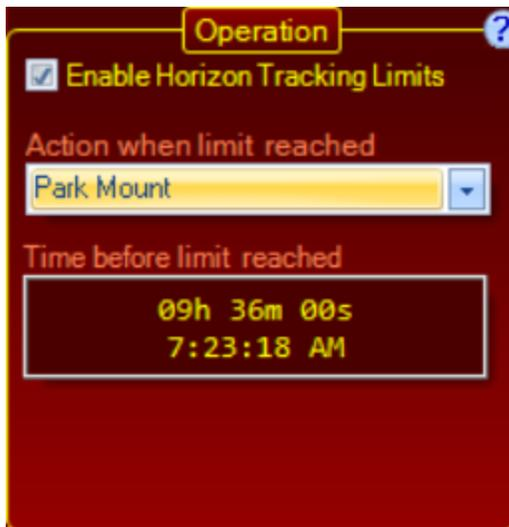
**Action when limit is reached:** Choices are **Stop Tracking**, **Park Mount** or **Just Warn**. If Park Mount is selected, APCC will park to the park position selected on the [Park tab](#). When the limit is reached, the Horizon Limits Indicator in the Telescope Position section of the main window will begin to flash alternatively between the dark red and yellow
