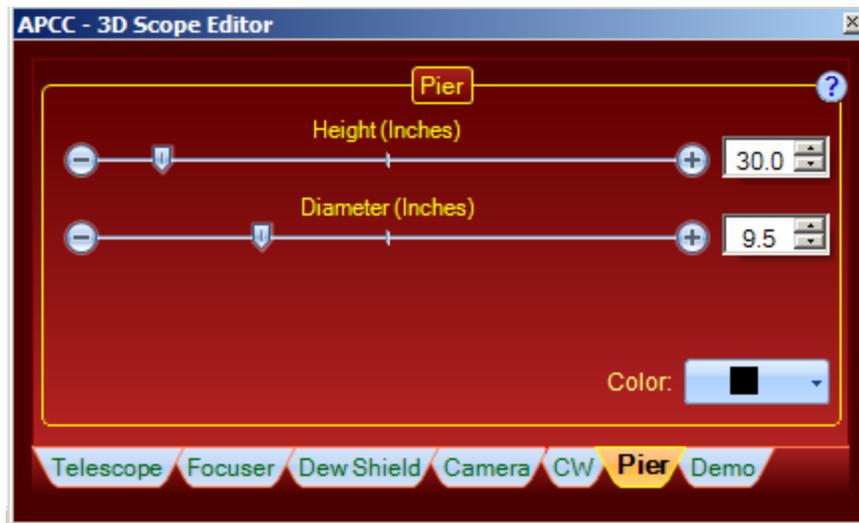
**Height, Diameter:** Adjust dimensions with slider, arrows or number entry. Consider entering a lower pier height since entry of larger numbers may push the scope out of the view. Unless your telescope is so long it might strike the floor, this is not an important parameter of your setup.
