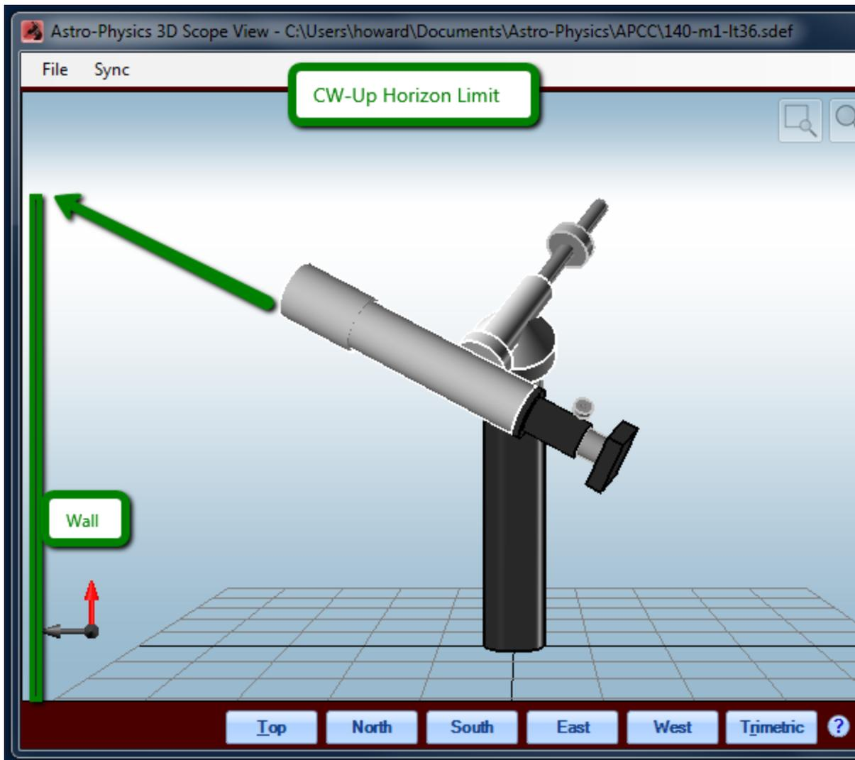
The **Meridian Tracking Limits Explorer** helps you setup custom meridian tracking limits for each declination. You record a series of limit values, and the Explorer interpolates a full curve from these points to give you defined limits throughout the sky. The Meridian Tracking Limits Explorer Window is shown below. To access this screen, click on Edit to the lower right of center on the Meridian Tab.
