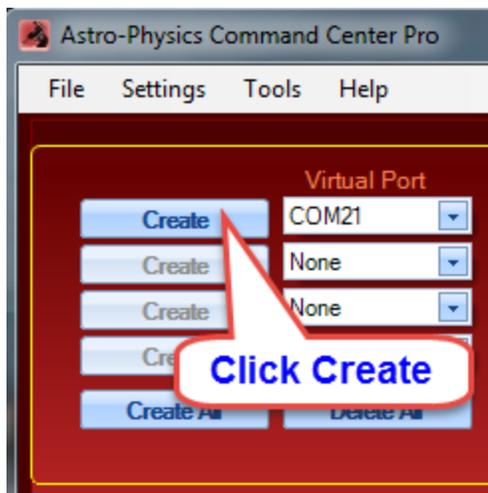
7. Repeat this for the second COM port (i.e. COM 22) and any additional ports you may need. Defining the second port is recommended so that ASCOM client programs that must be run as administrator can have their own instance of the driver.
