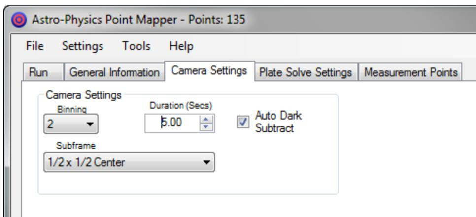
**Binning:** Select your camera binning here. Camera binning groups pixels together to provide greater signal to noise. 1x1 binning doesn't do any grouping. 2x binning groups four pixels (2x2) into one large pixel. If your image scale when binned is less than 3 arc-seconds/binning pixel then plate solve accuracy will not be affected. For more information on binning see this link: <http://www.ccd.com/ccd103.html>
