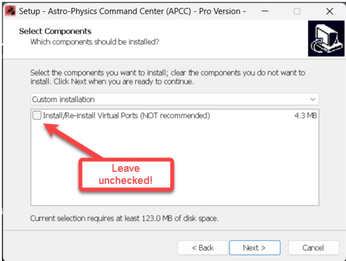
Installation Screen Capture. We no longer recommend installing the Virtual Ports.
