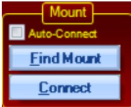
**Auto-Connect** - When this is checked, APCC will attempt to connect to the mount as a part of its start-up sequence. **If you have this box checked, you will want to have an overall start-up procedure that powers the mount ON before starting APCC.** This is common practice and is recommended in permanent and remote systems. Once connected, APCC will proceed through the initialization procedure you have previously defined.
