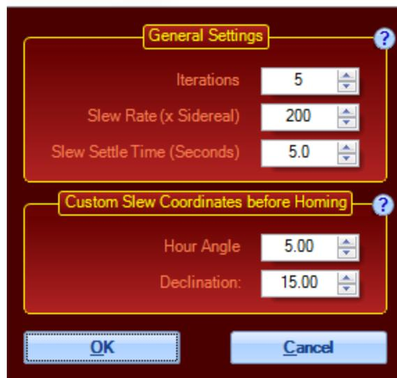
**Iterations:** This is the number of homing slews that will be used to create the average value in the Establish Home routine. Five iterations is a good value to use with three being the minimum number of iterations that we would recommend. This setting does NOT apply to the Find Home routine.
