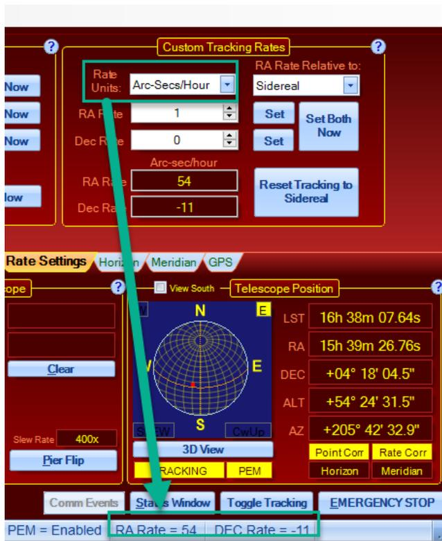
APCC Pro - The displayed RA rate units is now Arc-sec/hour in the **Tracking Correction Status** group box on the **Pointing Model** tab. Hovering the mouse over the box will show the old value (Sec/hour).
