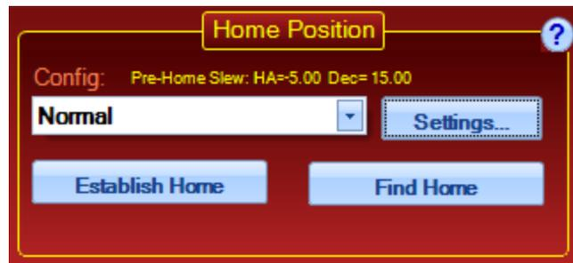
**Config Drop-down Box:** This selection tells APCC whether your telescope is set up in the conventional orientation (Home roughly equivalent to the AP Park 2 position) or in a side-by-side setup (Home roughly equivalent to Park 3). A third "Custom" setting is also available. This configuration then provides you with default values for the settings described immediately below.
