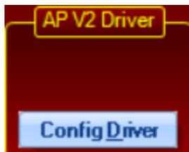
**Config Driver** - When this is pressed, APCC will try a one-time configuration of the relevant sections of the AP V2 Driver's settings in order for the driver to connect properly.
