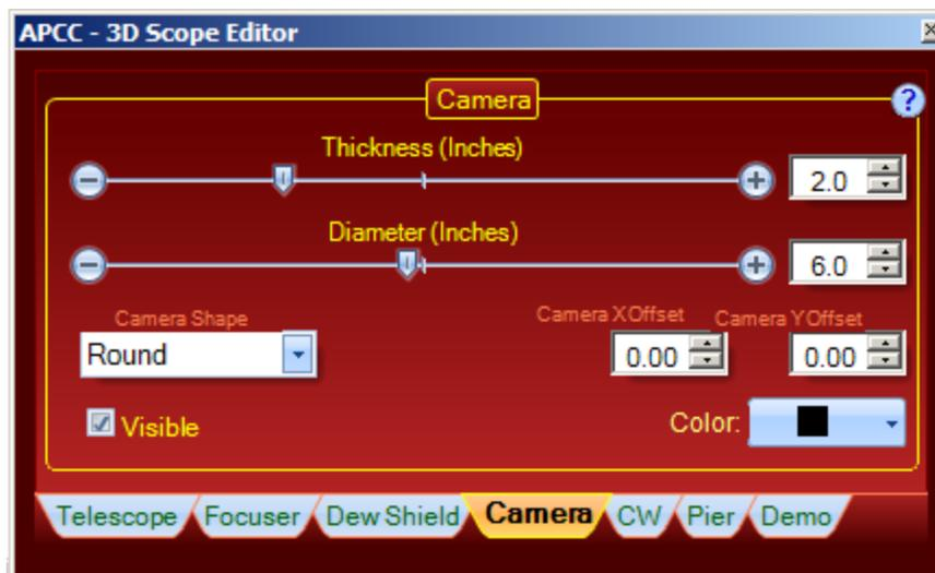
**Thickness, Diameter:** Adjust dimensions with slider, arrows or number entry.
