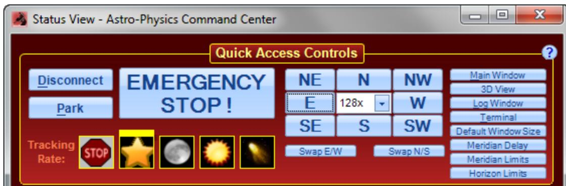
**Connect / Disconnect:** To connect APCC to your mount, press this button. Note that if an ASCOM application invokes the driver and the driver cannot connect to APCC on its virtual port then the driver will try to start a new instance of APCC and wait until the connection has been established. In the Connection Group box, you will want to have "Auto-connect when started" checked. Refer to [Connection Group Box](#) for more information.
