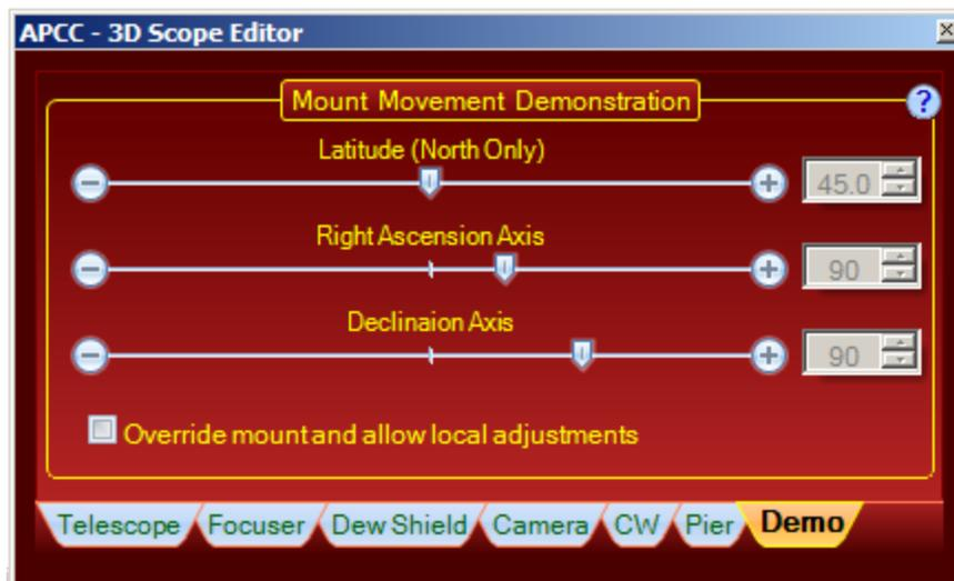
This Demo window allows you to experiment with latitude, RA and Dec values to create a graphic model without actually moving the scope to a particular position. This feature has been useful for us to create graphics.
