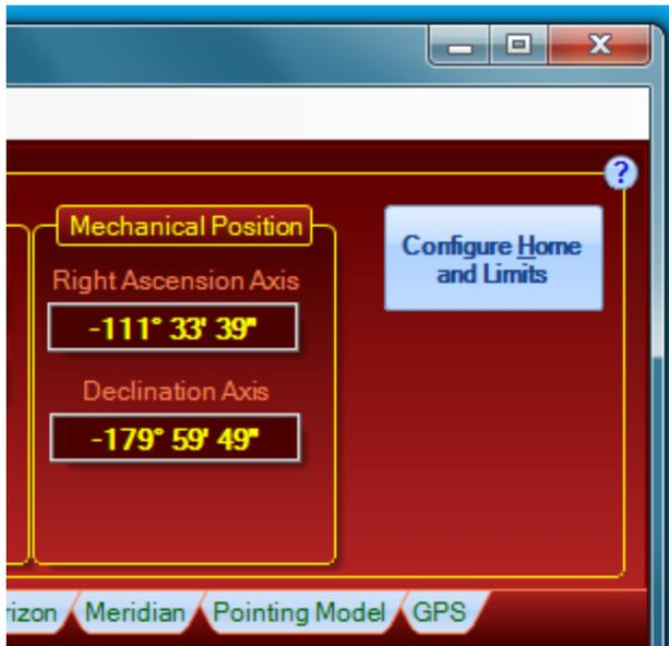
The Mechanical Position box tells you the current distance in degrees, minutes and seconds from the defined Home position. These values are especially useful when you define Home to be at Park 3, with the counterweight shaft pointing down and the scope pointing at the pole. For other home positions, you may need to do a bit of mental arithmetic to relate to the mechanical position.
