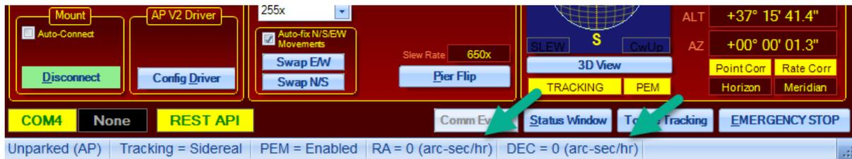
APCC - Fixed RA and Dec tracking rates displayed in the Status window.
