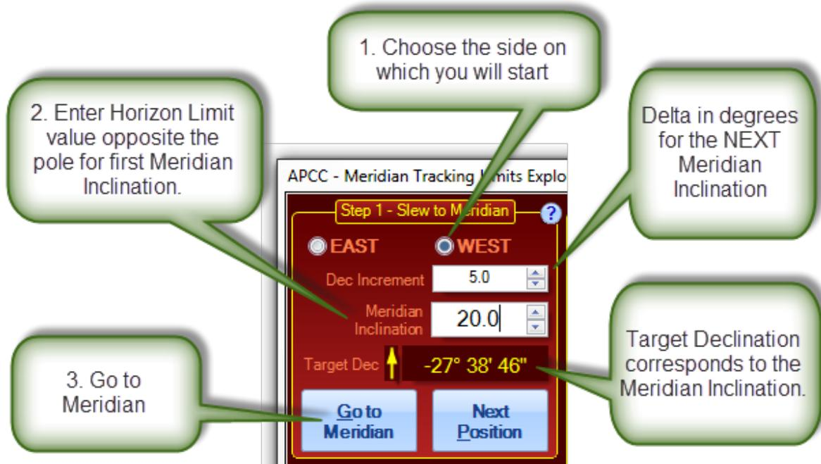
4. For this first point, DO NOT move the mount further with the E-W buttons. Instead, simply click the "Add Point" button at the bottom of the Step 2 box.
