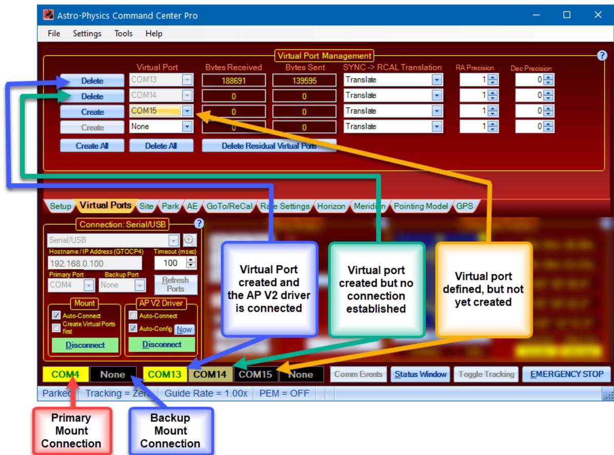
**Create:** Creates a virtual port when clicked. You must have an available port selected from the corresponding Virtual Port dropdown list. Once a virtual port is created, its color changes to a dim yellow with black letters and this button changes to *Delete*. **YOU MUST click the "Create" button to create the port in your system!** This isn't simply an APCC option, but goes to the heart of the PC's operating system.
