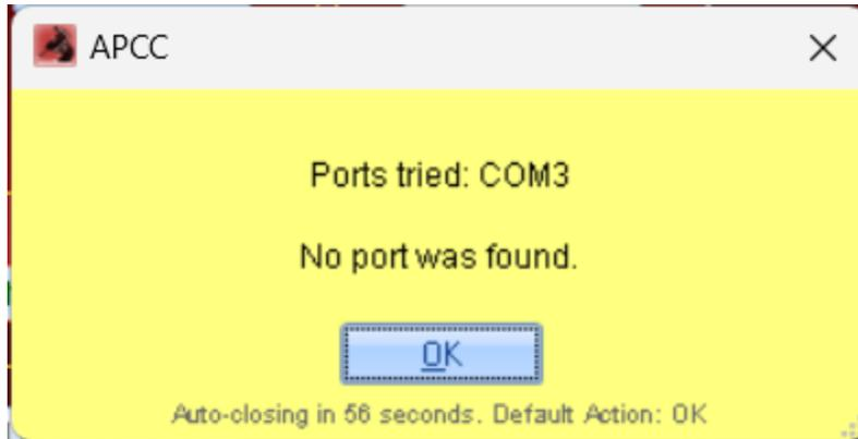
At this point you will need to investigate the physical mount connection (USB cable) and/or confirm the proper FTDI drivers are installed.
