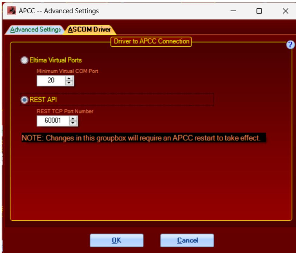
**Eltima Virtual Ports:** When selected, Virtual Ports will be used when the ASCOM driver is connected to APCC. The default and recommended setting is to use REST API instead of Virtual Ports
