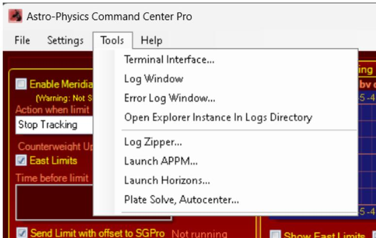
**Terminal interface...:** This opens the Terminal Interface window, which allows you to manually send commands directly to the mount. Please see [the Terminal Interface Window section](#) for more details. The Terminal Interface Window can also be accessed from a button on the [Setup Tab](#).
